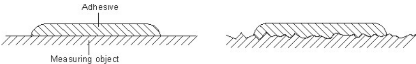
Fig. 2.3-1: Influence of surface roughness on efficient contact area
